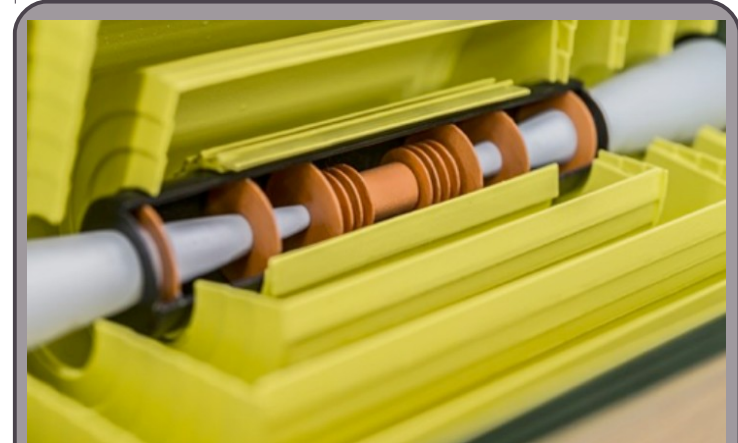
Multi-layer barrel and endcap pixel detectors (560 mm in length, Barrel radius from 30 mm to \sim 70 mm)
