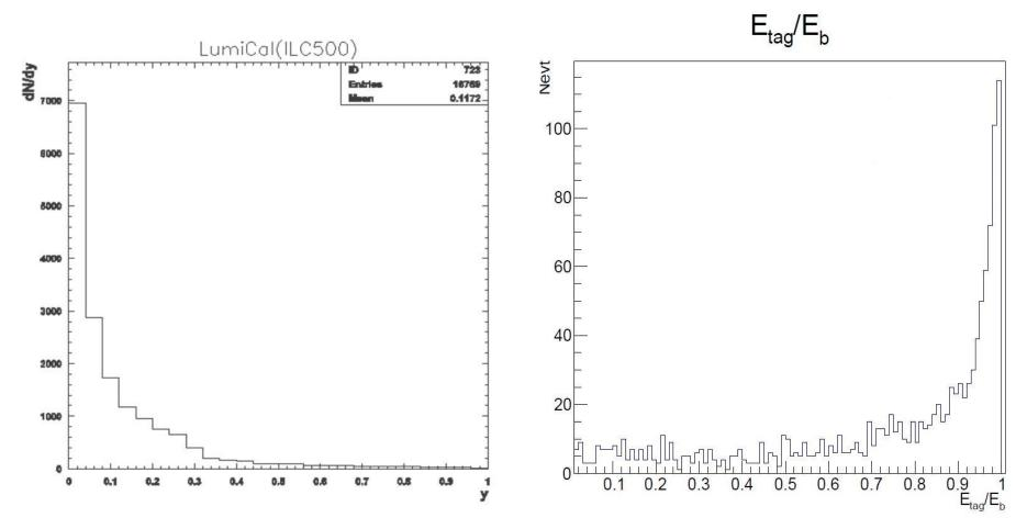
For LumiCal, the accepted angular range cover 31-78 mrad and the mean value of y is less than  $0.12 \implies \mathbf{F}^{\gamma}_{\mathsf{L}}$  term can be neglected.
