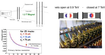
tracking:  $\delta p/p \sim 0.45\%$  - reconstruction efficiency  $\sim 95\%$  for  $p > 5 \, GeV$ . Data taken with two magnet polarizaties.
