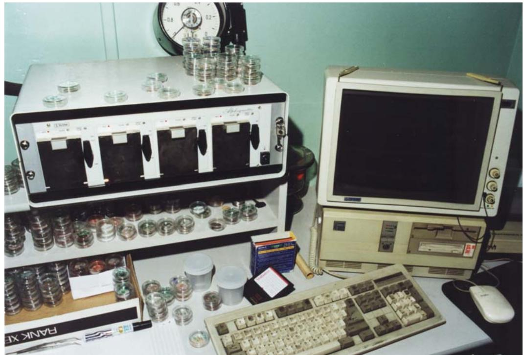
Alpha spectrometer Silena AlphaQuattro (4 tracks), PIPS and SBSi detectors
